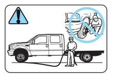
**WARNING** An inflated tire and rim can be very dangerous if improperly used, serviced or maintained. To avoid serious injury, never attempt to re-inflate a tire which has been run flat or seriously under-inflated without first removing the tire from the wheel assembly for inspection. Do not attempt to add air to tires or replace tires or wheels without first taking precautions to protect persons and property.
